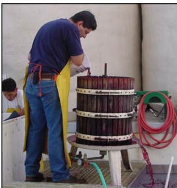
Pressing is still done in an old style basket press.
