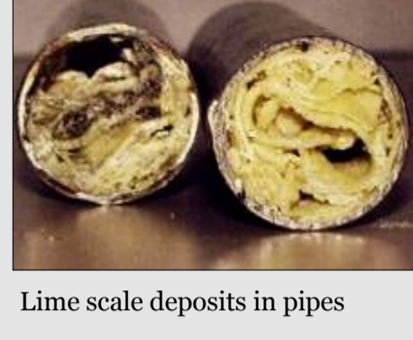
Lime scale deposits in pipes
